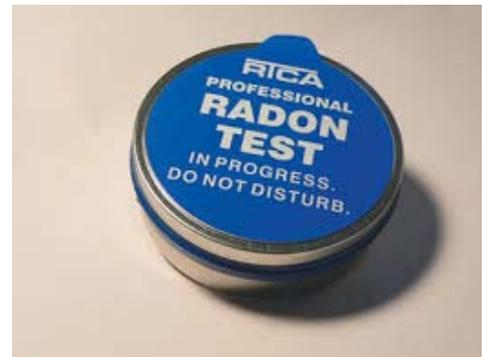
Two weeks after the notification has been sent out, 3-inch passive diffusion charcoal canisters are placed in all of the frequently occupied classrooms that are in contact with the ground. They are left in place for approximately three days. Once they are retrieved, they are immediately sent to a certified lab for analysis.
