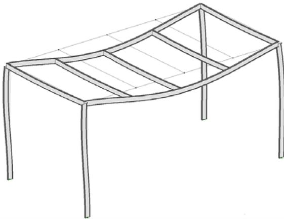
**Figure 1:** Exaggerated deflection of structural elements.
